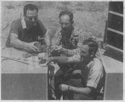
INSTRUMENTATION equipment to record blast effects on a model three-story building is installed by (1 to r) Tom Vance, Bob Foster and George Burnside, of the Coyote Canyon Section.
